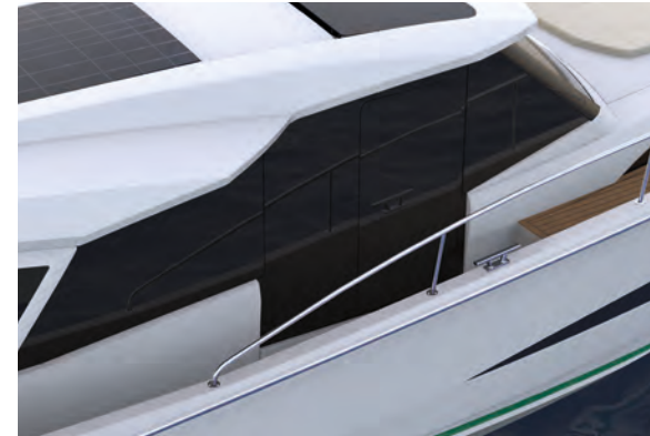
A wider asymmetrical side deck to starboard has a sliding door to the helm station for easy access during navigation, anchoring or docking.
