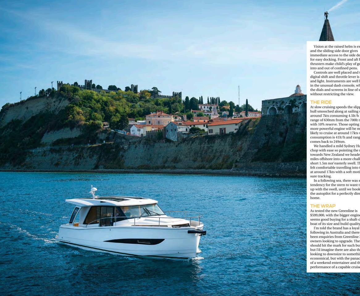
Vision at the raised helm is excellent, and the sliding side door gives immediate access to the side deck for easy docking. Front and aft bow thrusters make child's play of getting into and out of confined pens.
