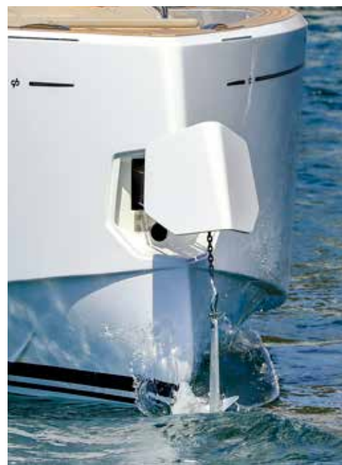
Below: A cleverly designed hatch in the bow opens for anchoring access.
