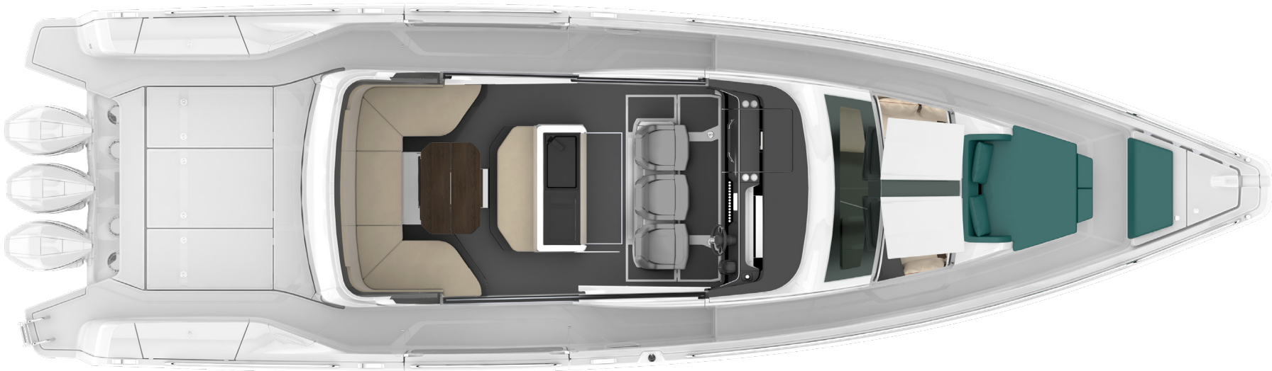
Rendering above showing the Axopar 45 Cross Cabin layout with standard aft deck and wetbar center piece in full forward position.
