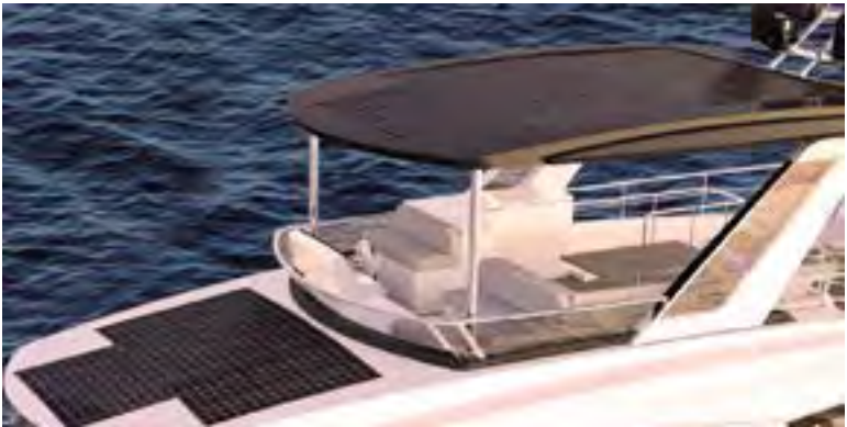
☀️ 11 solar panels | 3.6kW of solar power | Boat's domestic services to run without a noisy diesel generator
