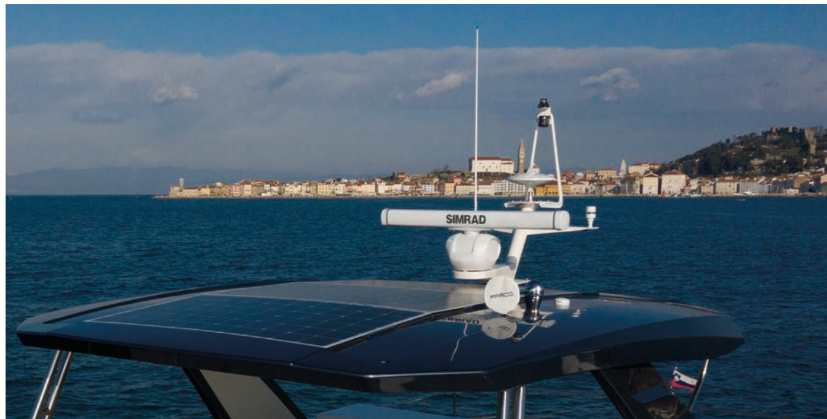
Hard-top incl. solar panels and HALO radar
