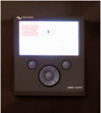
Control panel for tanks and electrical consumers
