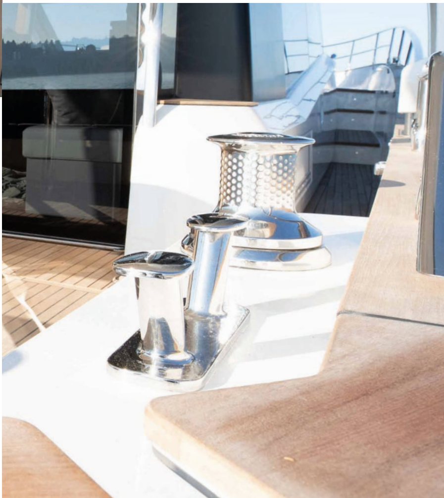
2 electric capstans aft for handling of aft mooring lines with foot controls
